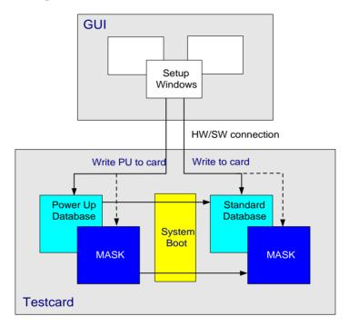
For both databases you can determine freely, which bits are fixed and which can be modified by BIOS or other program routines. This information is stored in the masks.
