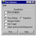
**2** Select the testcard components to be started when using the Run button or the Start item from the Run menu.
