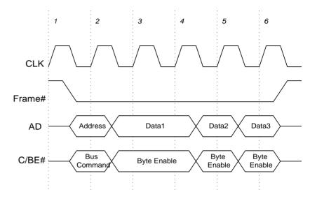
The figure shows a typical transaction, consisting of one address phase and one or more data phases.
