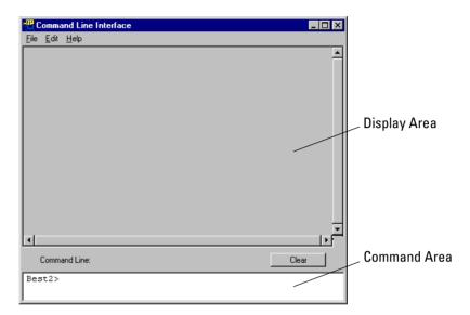
The Command Line Interface window is divided into two areas: The display area and the command area. The CLI commands (or their abbreviations) are entered in the command area and executed with the return key. The commands and the system responses are then listed in the display area.
