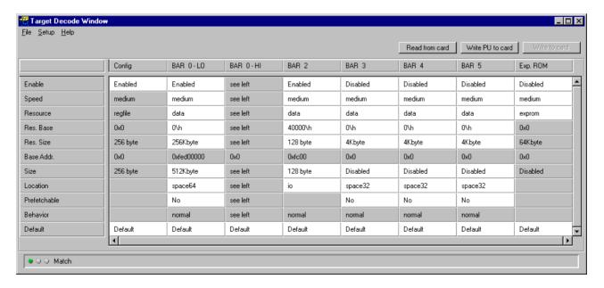
The columns of this window contain the settings for the configuration decoder, the six standard decoders, and the expansion ROM decoder (from left to right).
