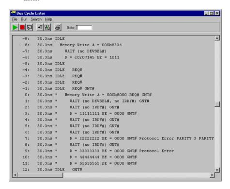
Note that two protocol violations are indicated. If the tool was connected to an actual testcard, examining the Protocol Check window would reveal that the second protocol violation indicates that a parity error occurred but was not signaled by the receiver of the data.
