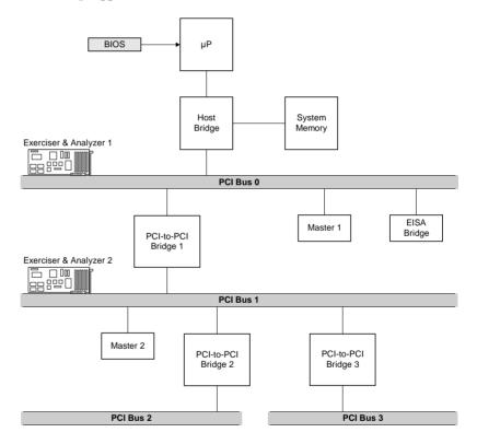
You can use the Exerciser's master and target features to test each individual device—or the system as a whole:
