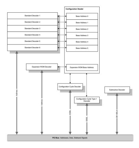
The transactions to be claimed by each decoder are specified by the base addresses (see "Base Address" on page 60).
