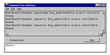
Call three commands were typed in at the *Best2>* prompt. The commands are displayed along with the results in the output area of this window. In this case no specific output was returned by the testcard. Hence, only *ready* is displayed to indicate successful completion of the command.
