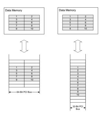
To align the data correctly for data transfers to or from the PCI bus, follow the rules below.
