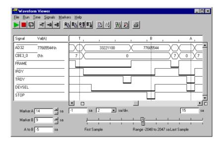
Notice that the PCI Exerciser target behaves exactly as it was set up:
