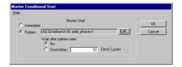
In this dialog box the pattern is set to start the transactions after an access to the address range  $b8000\h...b8fff\h$  is done. This is coded in the boolean expression next to the *Pattern* radio button. To start the master transactions, both the value of the AD32 bit vector must be  $b8xxx\h$  and it must be an address phase at the same time.
