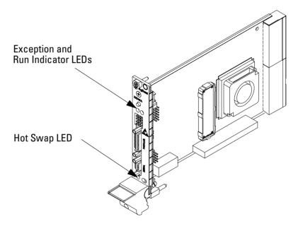
When inserting the testcard, the blue LED will light up as soon as the testcard is powered. After successful hardware and software layer connection, the LED will turn off.
