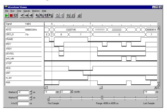
Note the transaction that triggers the start of the Exerciser (shown at marker A). It is also easy to identify the transaction block during which the master is active (m\_act is high from the trigger point T on; it is always high while the testcard's master is active). During this time the AD32 signal first holds the target address (address phase) and then the transferred data in the five data phases.
